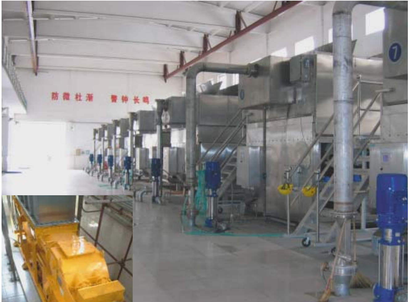
Dewatering building with locally produced belt filter presses
